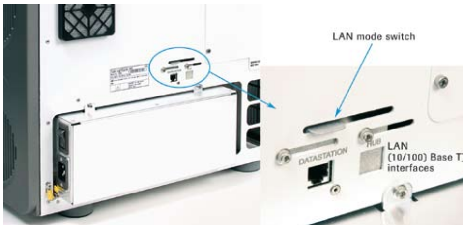
Figure 5 LAN interface at the rear side of the instrument
