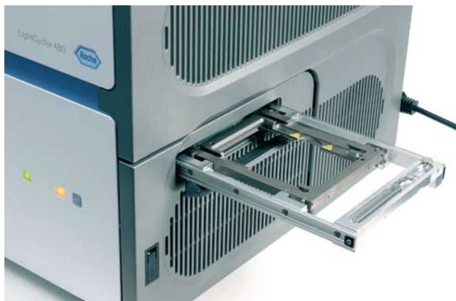
Figure 10 View of an ejected multiwell plate loader
